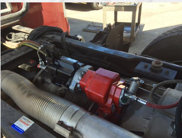
— HYDRAULIC PUMP — MOUNTED ON THE PTO
