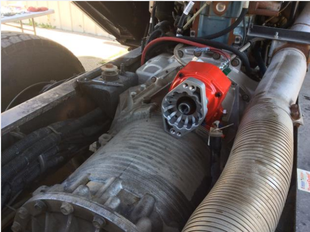
— POWER TAKE OFF (PTO) — ON THE POWER TRAIN
