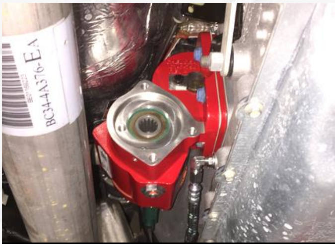
PTO BOLTED TO TRANSMISSION
