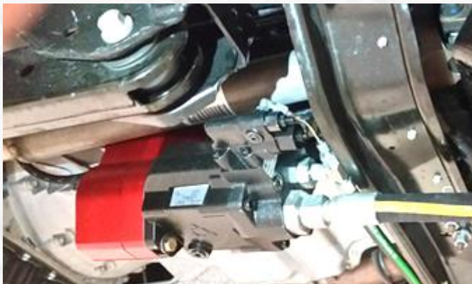
PUMP BOLTED TO HYDRA-DRIVE
